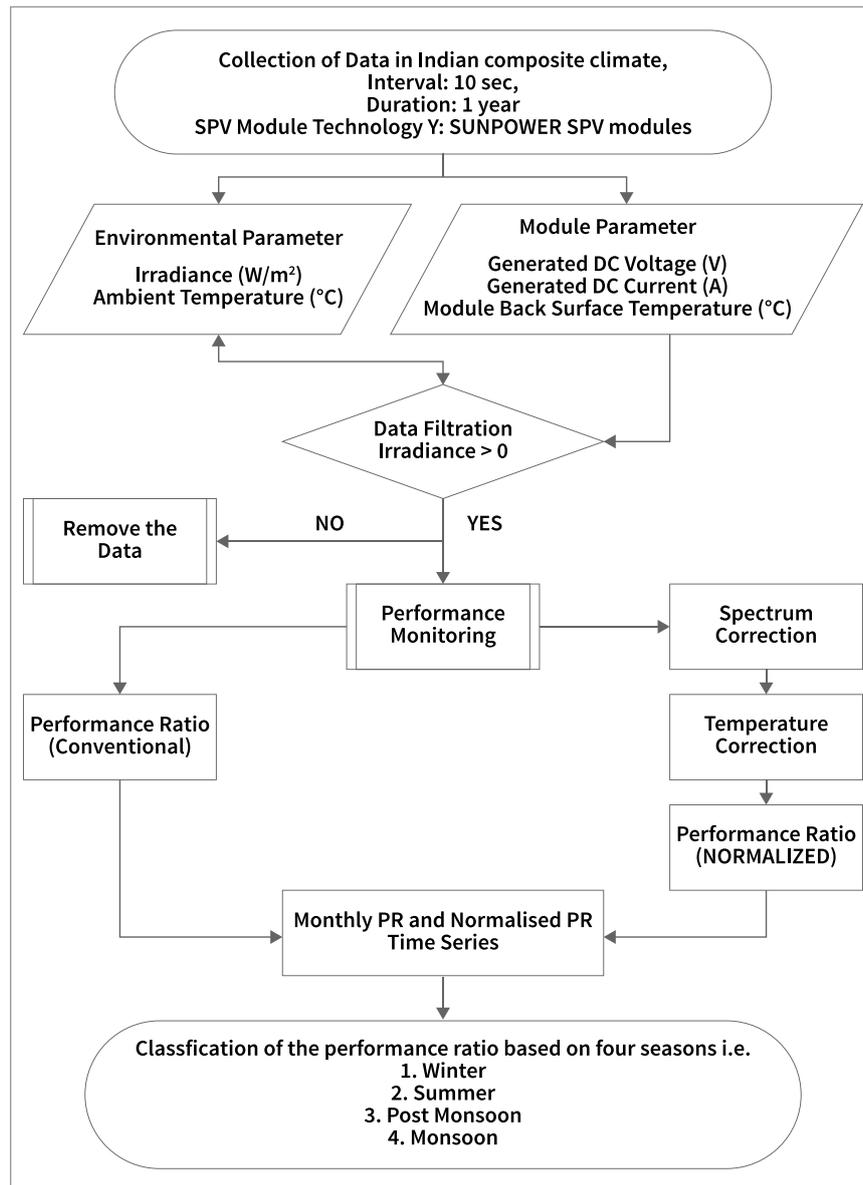
FIGURE 2. Flow-chart of the procedure followed for the performance monitoring
